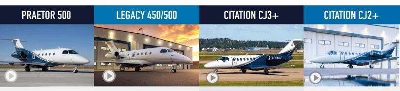
8/9 Passengers 45,000 ft Service Ceiling ProLine Fusion Avionics Coast-to-Coast Capabilities WiFi 7 Passengers 45,000 ft Service Ceiling Garmin G3000 Avionics XM Weather WiFi 7 Passengers 45,000 ft Service Ceiling Pro Line 21 Avionics XM Weather WiFi
